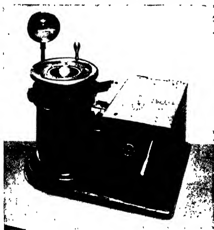
FIGURE 390. Two common types of cupping tests used on sheet metal to determine grain size and ductility.
